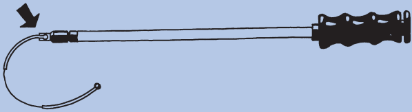
3. Screw the screw thread end of the Lap Loop electrode into the female thread at the distal tip of the introducer.
