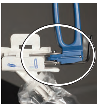
Photo 8 Pivot Point on the Handle lined up with the RUMI® II Manipulator Mating Hole in the Adapter
