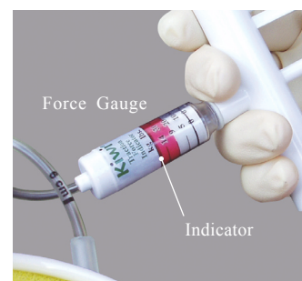
2 Indicator moves along gauge giving a force reading.
